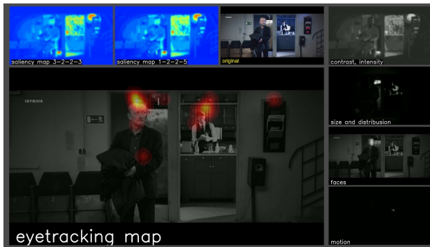
Figure 6: Right column (from top):. global contrast based saliency map, distance from center based saliency map, face presence based saliency map, motion based saliency map
