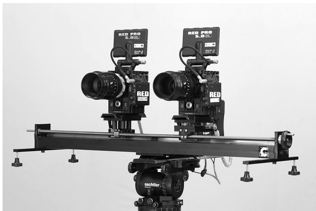
Figure 1: Parallel RIG equipped with two cameras [6]
